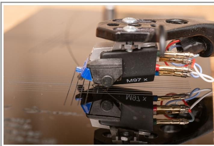
Finely adjust your arm's position until the cartridge's body is aligned with the grid lines,
