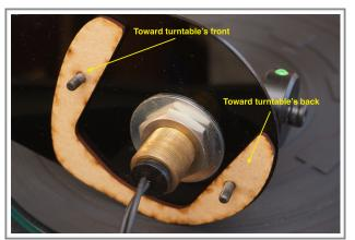
The spacers are not symmetric, study the pictures carefully to understand which is the right mounting side.
